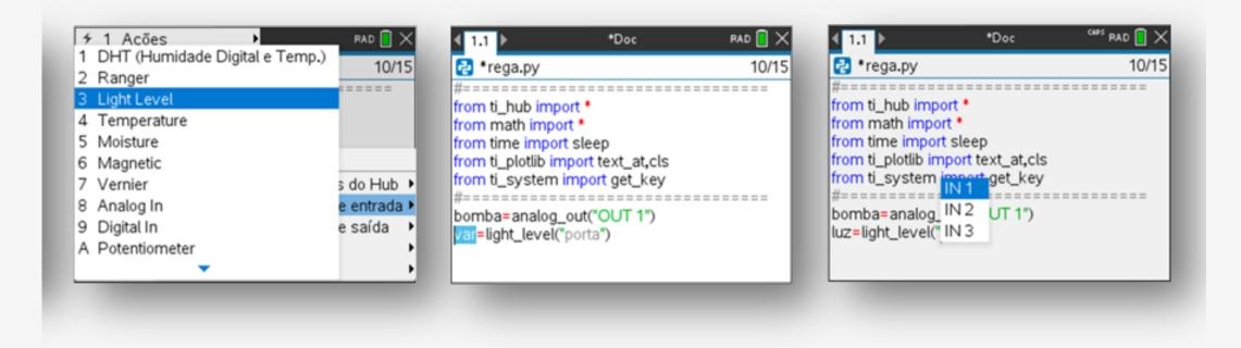
To see all the object luz commands, press . after entering its name. In this case, use the options range(min, max), to reset the sensor scale and measurement() to obtain the luminosity reading.
