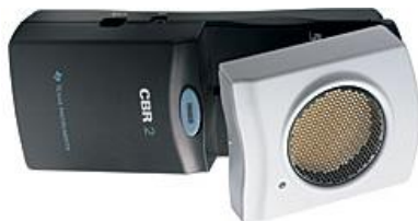
Figure 2 CBR-2 ultrasonic distance sensor
