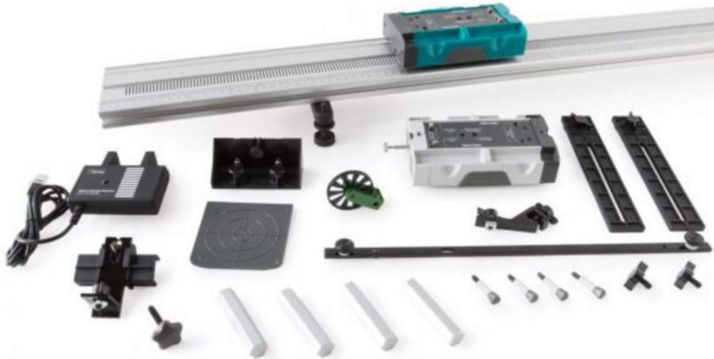
Figure 1 Dynamics Cart and Track System with Motion Encoder (Vernier)
