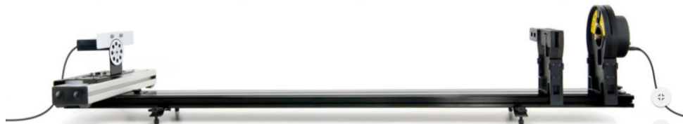
Figure 2 Experimental Setup. Left: position and intensity sensors , Right: slits-slider and laser
