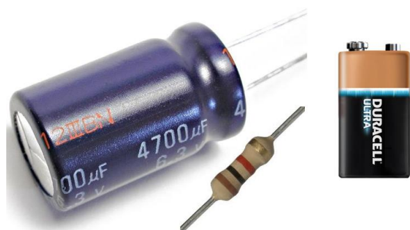
Figure 2 Electrolytic Capacitor ( 4'700 \mu\text{F} ), Resistor ( 1'000 \Omega ) and Battery (9 Volt)
