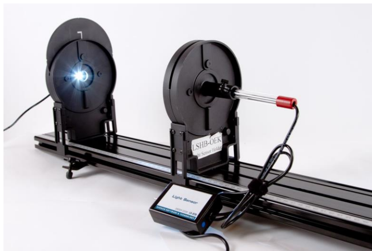
Figure 1 Experimental Setup: Track, LED Light Source, Light Sensor, Sensor Holder
