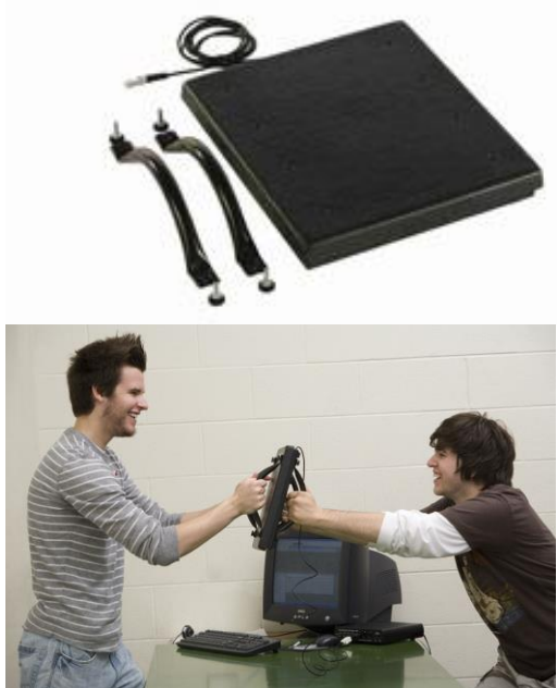
Figure 3 Vernier Force Plate: Newtons 3rd law
